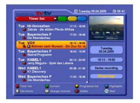
In the box at the bottom right of the screenshot above you see the day, date and time of recording and the recording mode. If two recordings overlap, the fact is indicated in the box at the bottom right.
